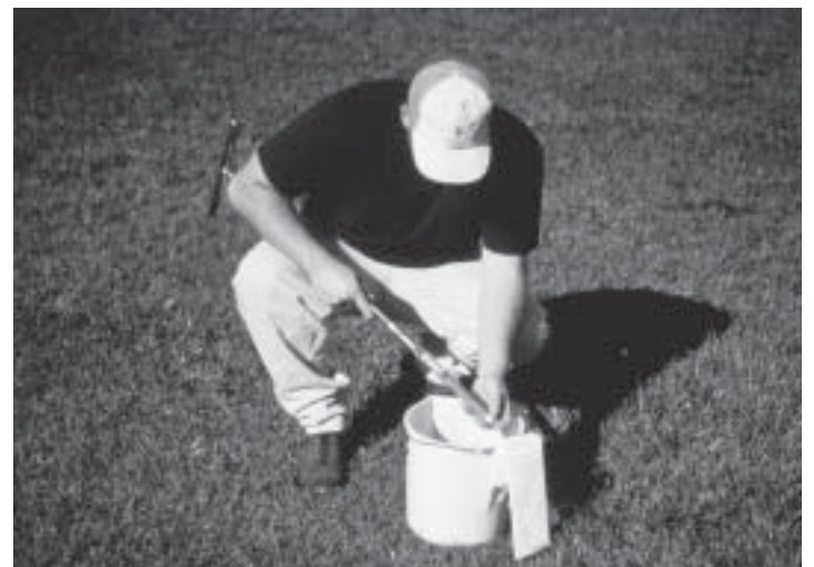
Figure 2. Penn State soil test sampling instructions suggest mixing all subsamples together to make one sample.
