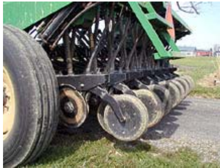
Fig. 8. Press wheels improve seed-to-soil contact. Photo by Marvin Hall.
